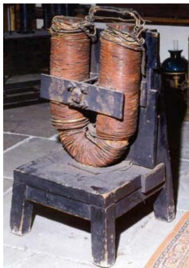
Fig 3.20 Faraday's giant electromagnet which he used in the diagrammatic experiments, 1840s-1850s. RIAC 00084
