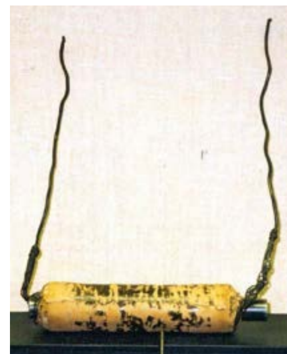
Fig 3.17 The first electric generator made by Faraday on 17 October 1831. RIAC 00022
