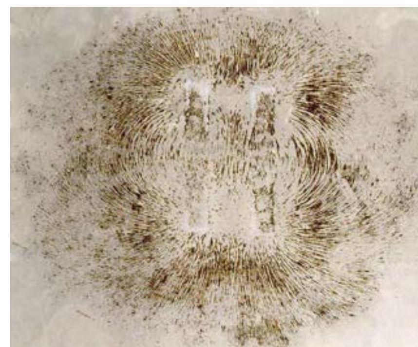
Fig 3.19 Iron filing diagrams made by Faraday c.1850 to illustrate that space had structure near a magnet. Ri Archival Collection
