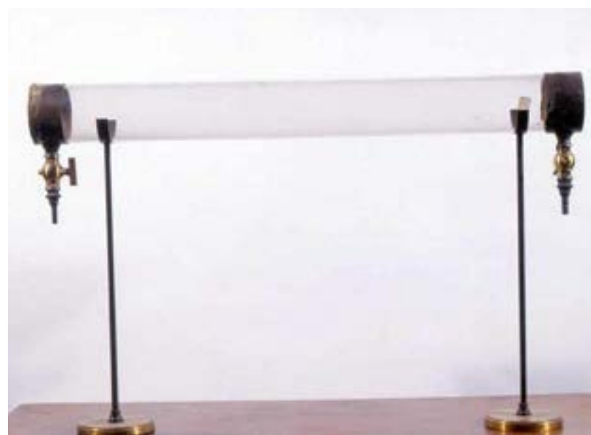
Fig 3.28 Tube which Tyndall used in his experiments on the scattering of light by particles, which led to his explanation of why the sky is blue. RIAC 00330c
