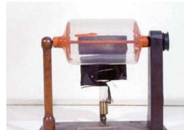
Fig 3.12 Faraday's electrostatic generator which he made while an apprentice bookbinder, c.1810. RIAC 0004
