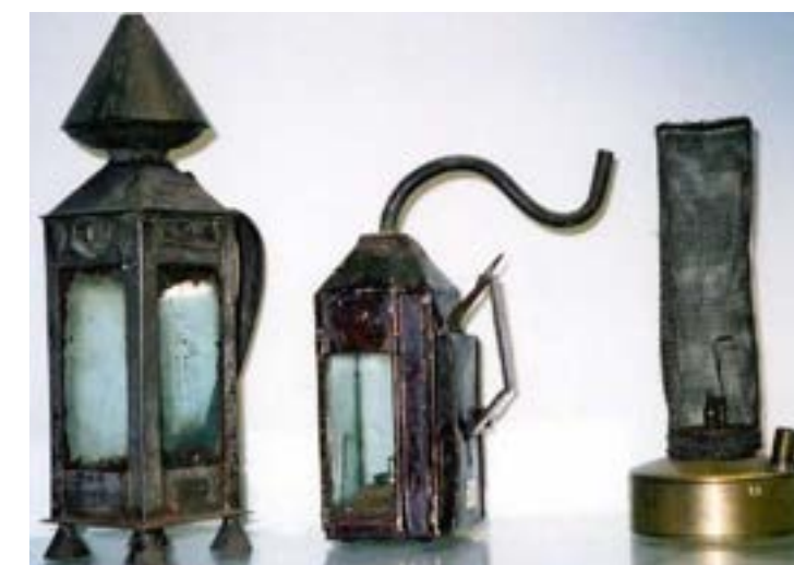
Fig 3.14 Some prototypes of Davy's miners' safety lamp
