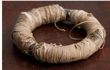
While Faraday describes the making of the ring in its entirety here, the actual work would probably have taken much longer. A modern experiment to build a replica induction ring using original materials took 10 working days.
